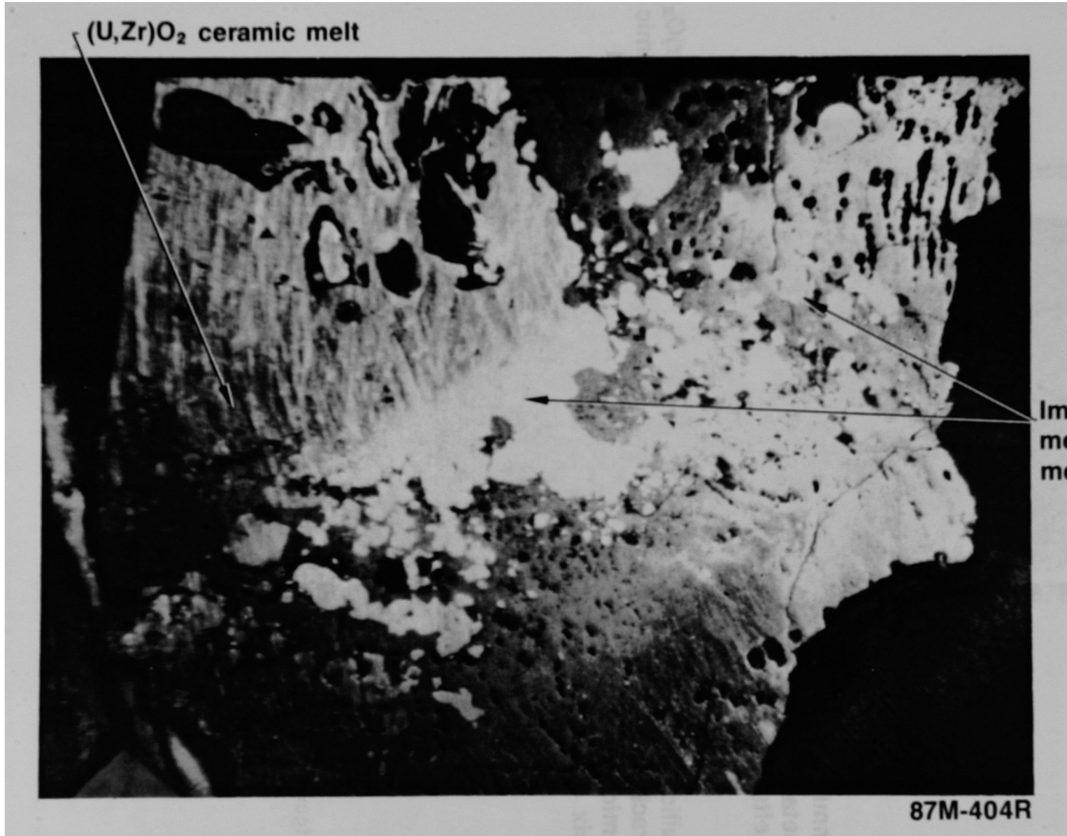
Figure 4. Cross section of upper crust from K09-P2.
